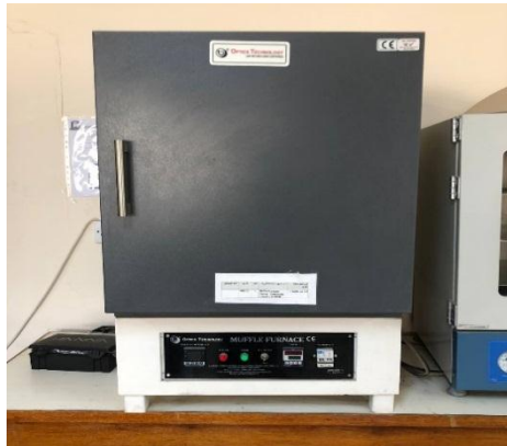
فرن حرق 1200م ( Muffle Furnace Optics ) (Technology)
